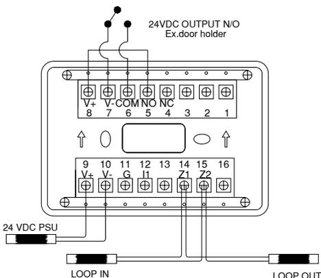
Wiring for 24VDC output
